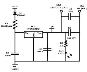
Figure 5: PLC Interface Equivalent Circuit
