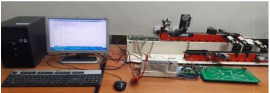
Figure 3: Experimental setup of Traffic signal control with PLC
