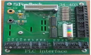
Figure 2: PLC Interface Module
