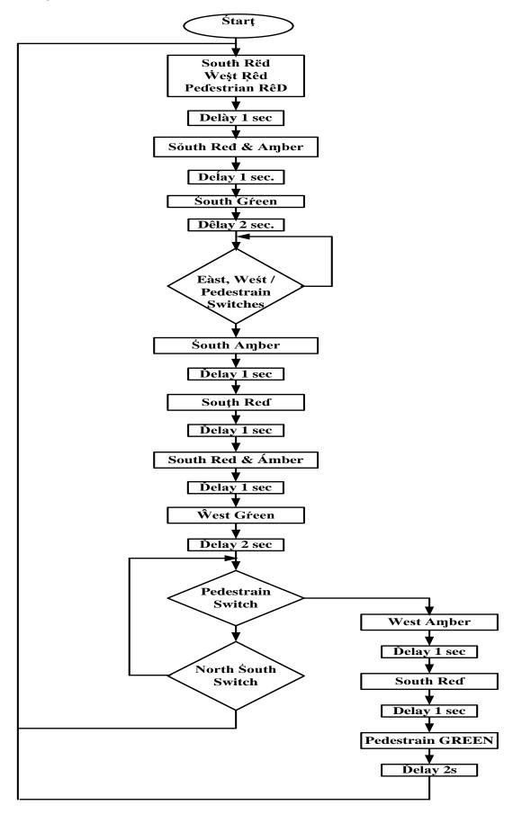
Figure 10: Flowchart of Traffic Light Control
