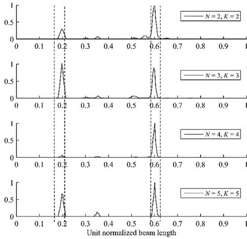
Fig. 10: Case2 estimated damage index -15% noise
