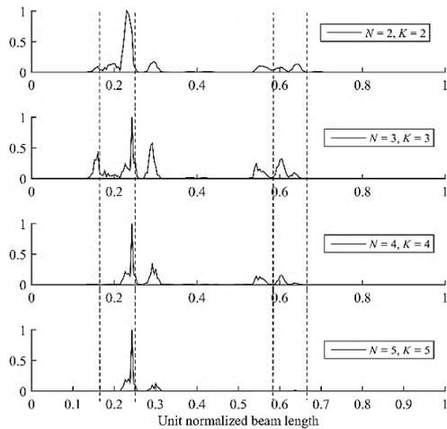
Fig. 6: Case1 estimated damage index - 15% noise
