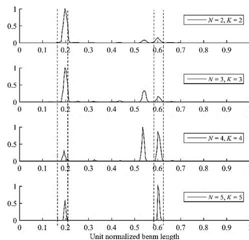
Fig. 9: Case2 estimated damage index - 10% noise
