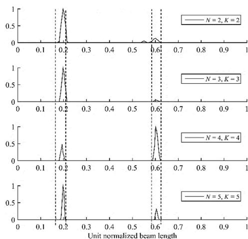
Fig. 8: Case2 estimated damage index - 5% noise
