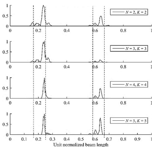
Fig. 4: Case1 estimated damage index - 5% noise
