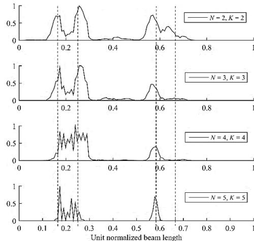
Fig. 5: Case1 estimated damage index - 10% noise
