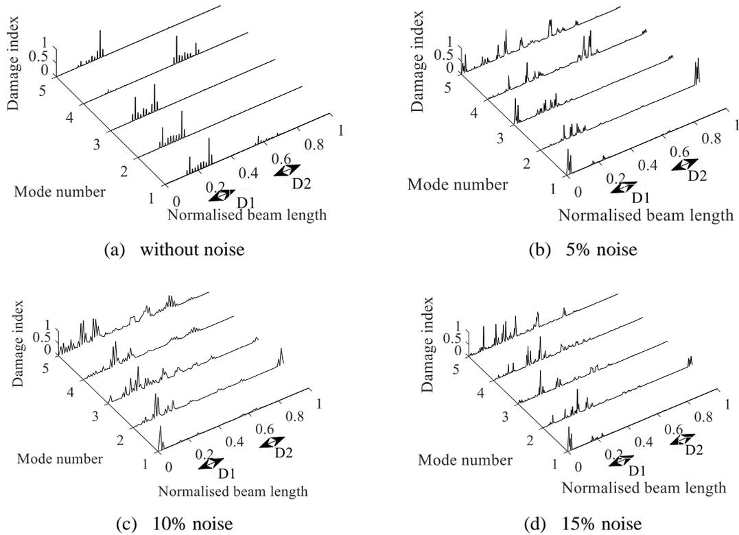
Fig. 3: Case1 damage indices from strain modes using GSM
