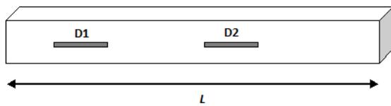
**Fig.1:** Beam schematic illustrating both delaminations
