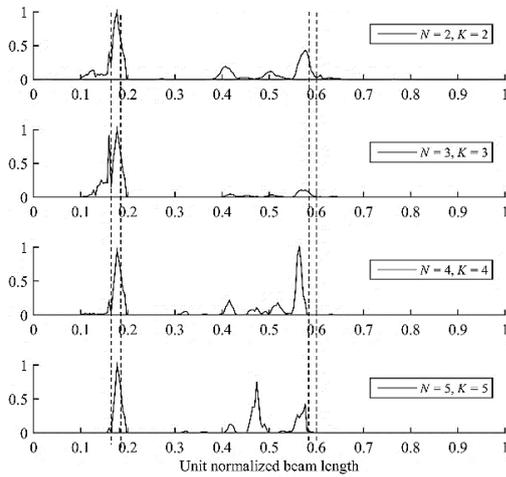
Fig. 12: Case3 estimated damage index - 5% noise
