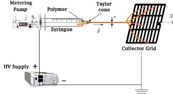
FIGURE 1. Electro-spinning process setup.
