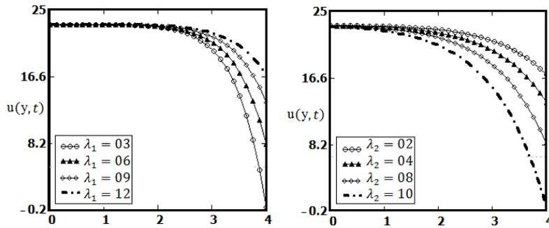
FIGURE 3. Profiles of the velocity field and shear stress for  $u_0 = 2, \Omega = 0.1, \nu = 8, \mu = 20, \lambda_3 = 18, \lambda_4 = 5.5, \Phi = 0.5, M = 0.2, \psi = 0.3$  with different values of  $\lambda_1$  and  $\lambda_2$ .
