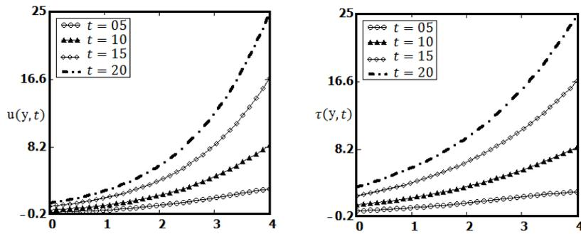
FIGURE 1. Profiles of the velocity field and shear stress for  $u_0 = 1, \Omega = 0.5, \nu = 0.679, \mu = 18, \lambda_1 = 0.7, \lambda_2 = 1.5, \lambda_3 = 4, \lambda_4 = 3.7, \Phi = 0.5, M = 0.2, \psi = 0.3$  with different values of  $t$ .
