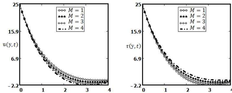
FIGURE 5. Profiles of the velocity field and shear stress for  $u_0 = 1, \Omega = 0.5, \nu = 0.679, \mu = 11, \lambda_1 = 0.5, \lambda_2 = 3.2, \lambda_3 = 9, \lambda_4 = 11.7\Phi = 0.5, \psi = 0.3$  with different values of  $M$ .
