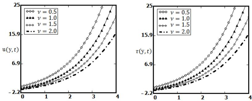
FIGURE 2. Profiles of the velocity field and shear stress for  $u_0 = 1, \Omega = 0.5, t = 5s, \mu = 12, \lambda_1 = 0.1, \lambda_2 = 1.1, \lambda_3 = 12, \lambda_4 = 6, \Phi = 0.5, M = 0.2, \psi = 0.3$  with different values of  $\nu$ .
