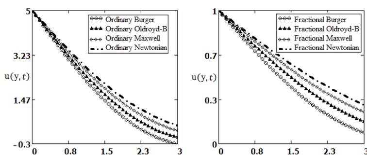
FIGURE 7. Comparison of velocity fields for four models for  $u_0 = 6$ ,  $\Omega = 0.5$ ,  $\nu = 1.679$ ,  $\mu = 11$ ,  $\lambda_1 = 4$ ,  $\lambda_2 = 9$ ,  $\lambda_3 = 11$ ,  $\lambda_4 = 20$ ,  $M = 2$ ,  $\Phi = 3.5$ .
