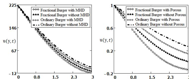
FIGURE 8. Comparison of velocity fields for four models with and without magnetic field and porous medium for  $u_0 = 6$ ,  $\Omega = 0.5$ ,  $\nu = 1.679$ ,  $\mu = 11$ ,  $\lambda_1 = 4$ ,  $\lambda_2 = 9$ ,  $\lambda_3 = 11$ ,  $\lambda_4 = 20$ .
