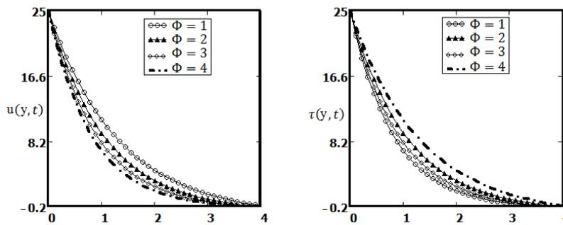
FIGURE 6. Profiles of the velocity field and shear stress for  $u_0 = 1, \Omega = 0.5, \nu = 0.679, \mu = 3.2, \lambda_1 = 2.9, \lambda_2 = 4, \lambda_3 = 25, \lambda_4 = 29.25, M = 1, \psi = 0.3$  with different values of  $\Phi$ .
