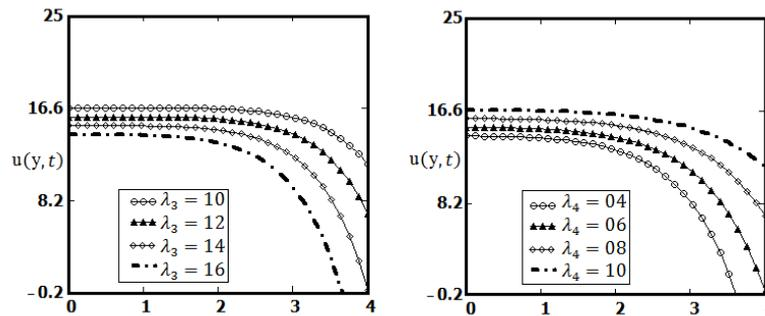
FIGURE 4. Profiles of the velocity field and shear stress for  $u_0 = 5, \Omega = 0.5, \nu = 25, \mu = 4.3, \lambda_1 = 0.7, \lambda_2 = 2.4, \Phi = 0.5, M = 0.2, \psi = 0.3$  with different values of  $\lambda_3$  and  $\lambda_4$ .
