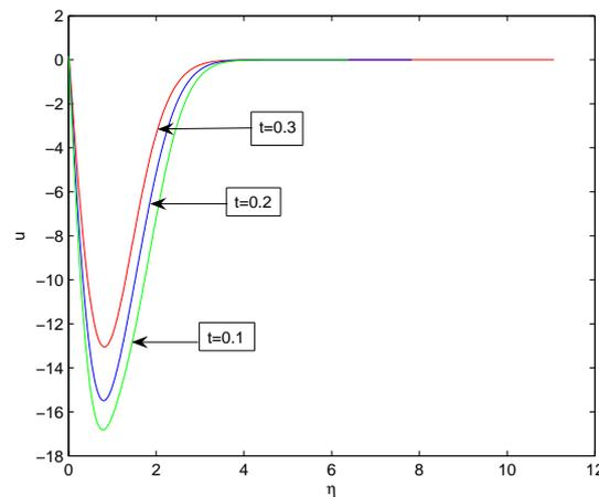
FIGURE 3. Profile of the expression for velocity given by Eq. (3.28) versus similarity parameter for  $Pr = 7$ ,  $K = 0.2$ ,  $\omega t = \pi/3$ ,  $Gr = 5$ ,  $Gc = 5$ ,  $Sr = 0.6$ ,  $a = 1$ ,  $b = 2$  and for different values of time.
