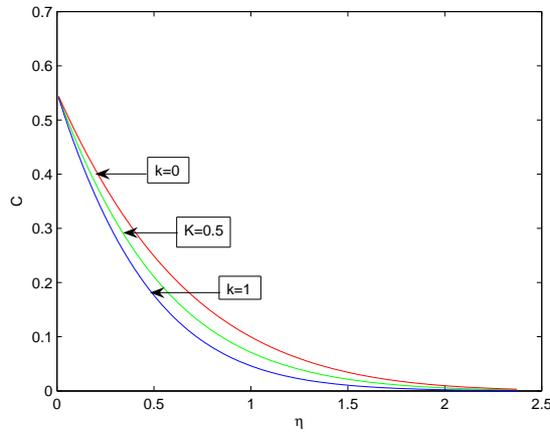
FIGURE 4. Profile of the expression for concentration given by Eq. (3.23) versus similarity parameter for  $Sc = 0.6$ ,  $t = 0.4$ ,  $a = 1$ ,  $b = 2$  and for different values of  $K$ .
