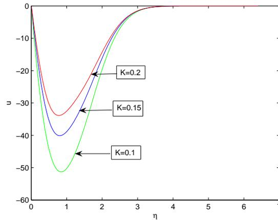
FIGURE 2. Profile of the expression for velocity given by Eq. (3.28) versus similarity parameter for  $Pr = 7$ ,  $Sc = 0.6$ ,  $t = 0.3$ ,  $\omega t = \pi/3$ ,  $Gr = 5$ ,  $Gc = 10$ ,  $a = 1$ ,  $b = 2$  and for different values of  $K$ .
