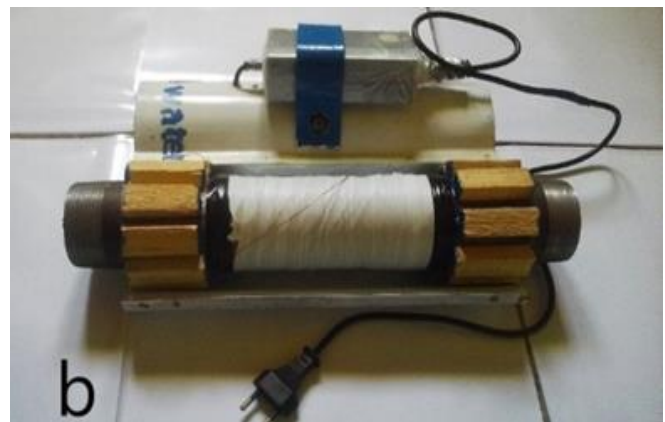
Figure 1. (b) the final fabricated magnetic unit.
