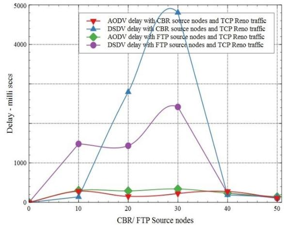
Figure 8. Delay with CBR/FTP source nodes and TCP Reno traffic type
