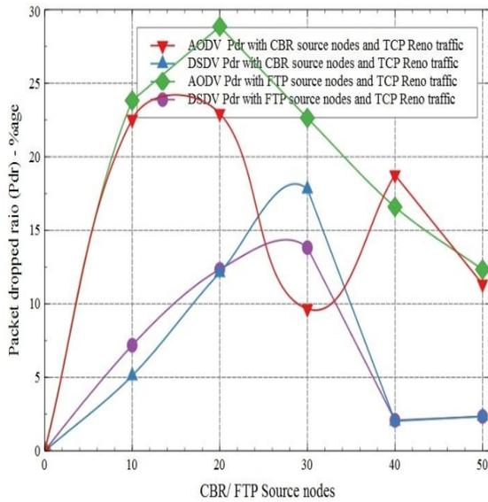
Figure 10. Pdrwith CBR/FTP source nodes and TCP Reno traffic type
