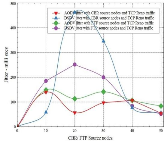
Figure 9. Jitter with CBR/FTP source nodes and TCP Reno traffic type
