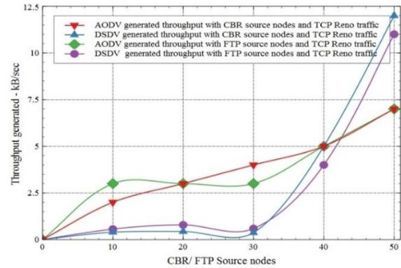
Figure 11. Generated throughput with CBR/FTP source nodes and TCP Reno traffic type
