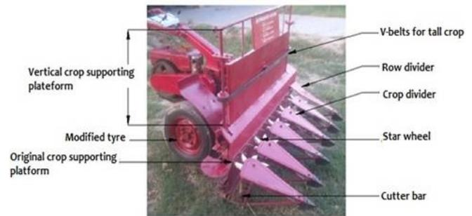
Figure 4. Improved design of engine operated reaper for tall crops in Engineering Workshop.
