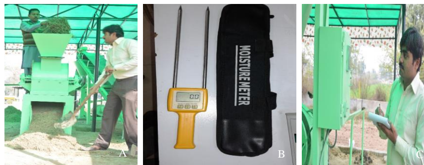
Figure 1. Machine/instrument used to determine operational parameters; A) shredder for required particle size, B) moisture meter to determine moisture content level C) electrical panel to note mould temperature (from right to left).
