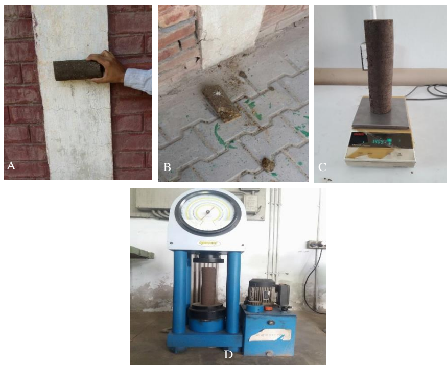
Figure 2. Determination of physical properties of briquettes A & B) durability, C) density D) compressive strength (from right to left).
