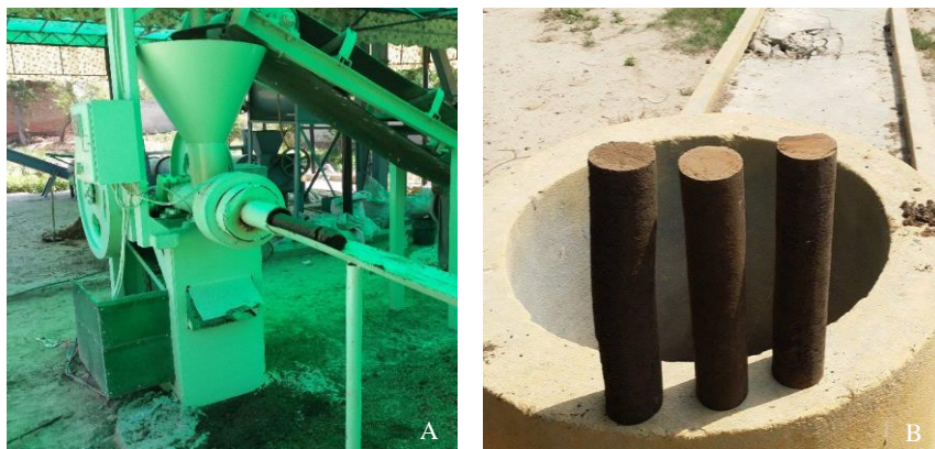
Figure 4. Preparation of briquettes using piston press briquettes machine.
