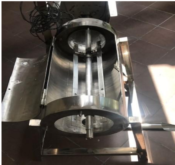
Figure 5. Beater shaft with incorporated teeth.
