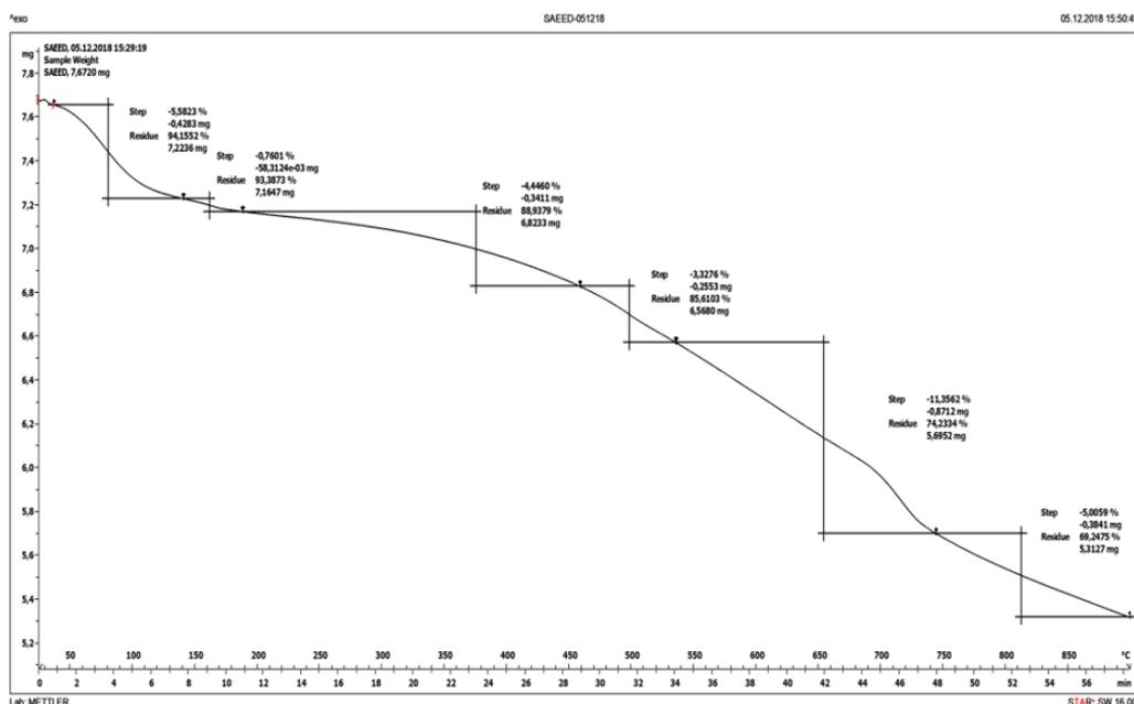
Figure 5. Thermogravimetric analysis (TGA) curve of biochar.
