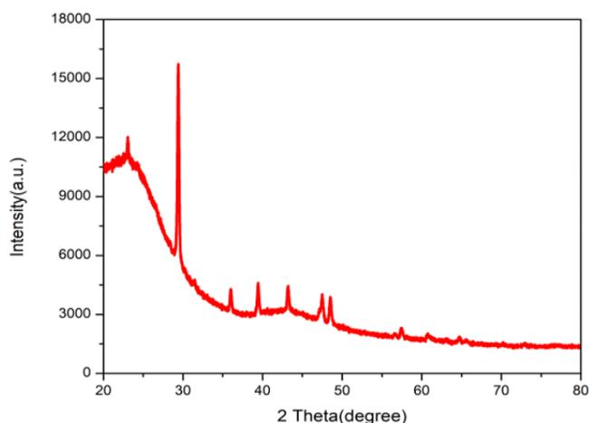
**Figure 2. The X-ray diffraction spectrum of produced biochar.**
