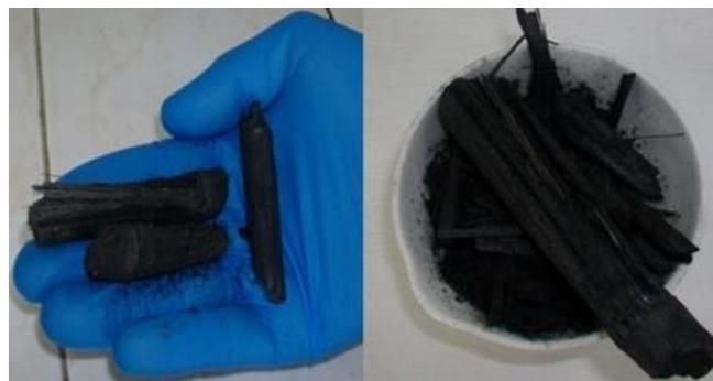
Figure 1. Production of biochar from maize at 700 °C.
