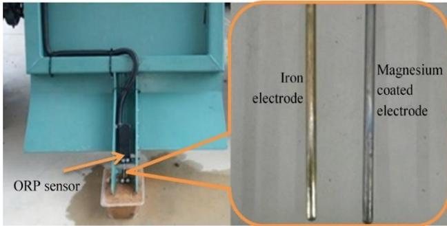
Figure 1. ORP sensor and its electrodes
