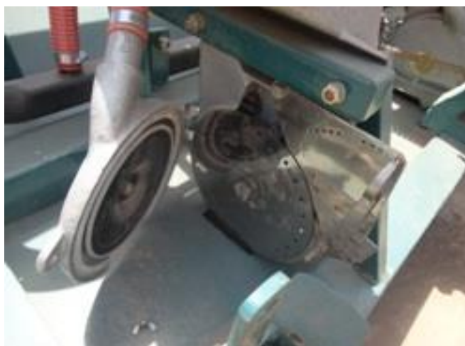
Figure 3. Pneumatic seed metering mechanism.
