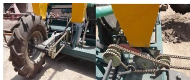
Figure 2. Power transmission to metering mechanisms using ground wheel and sprocket system.
