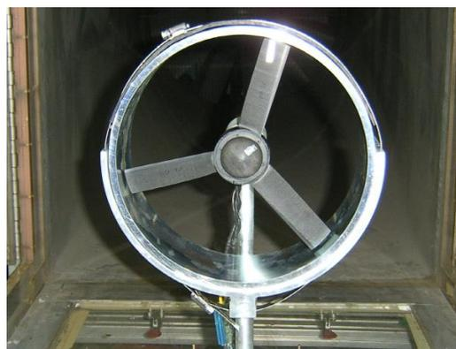
Fig 1: Ducted Fan Tested in AERO Lab
