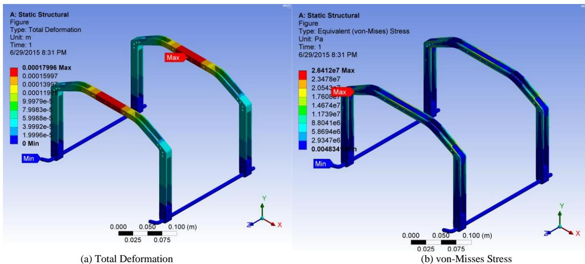
Fig. 3: Static structural analysis results for material combination1.
