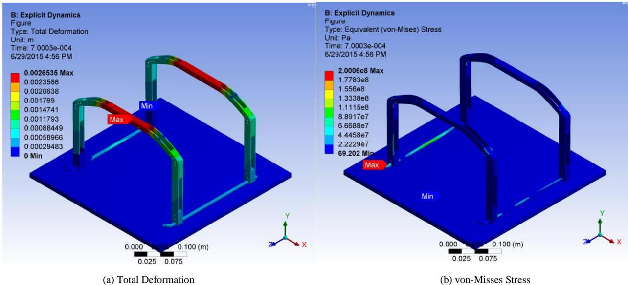
Fig. 6: Explicit dynamic analysis results for material combination2.
