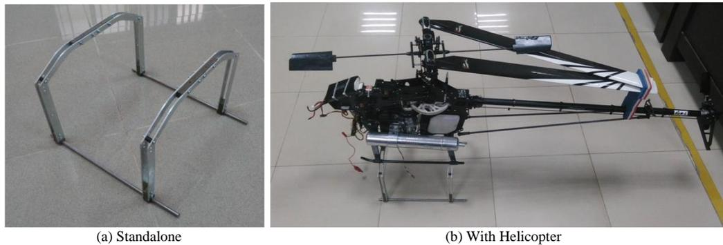
Fig. 7: Fabricated hardware assembly of proposed 195mm elevated skid design.
