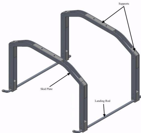
Fig. 2: Elevated Skid CAD Assembly.
