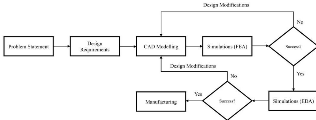
Fig. 1: Process flowchart for implementation of proposed elevated skid design.
