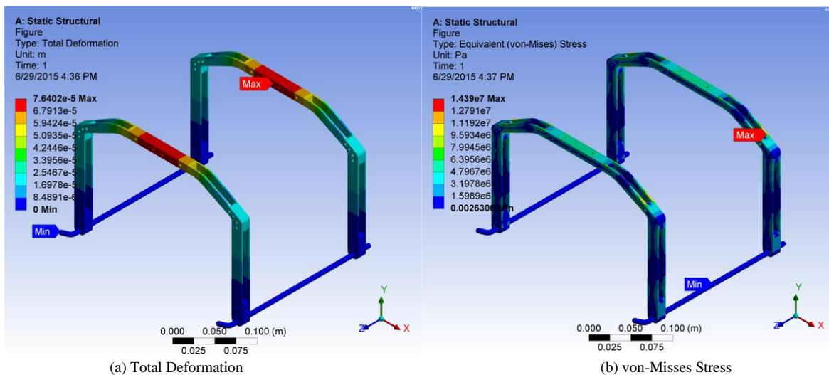
Fig. 4: Static structural analysis results for material combination2
