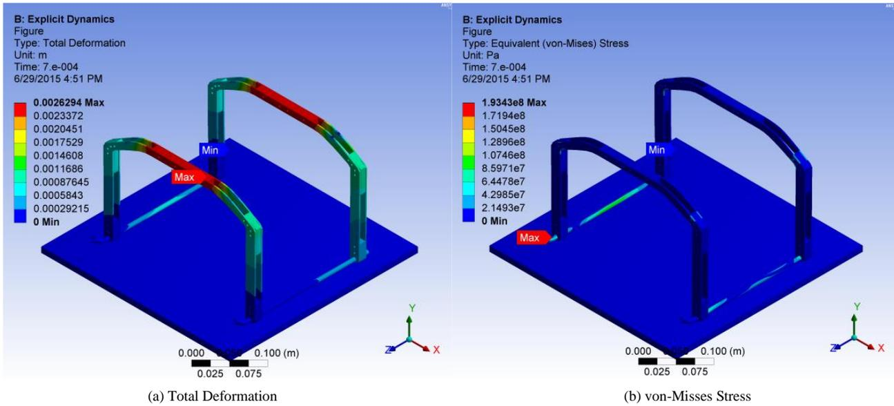
Fig. 5: Explicit dynamic analysis results for material combination1.
