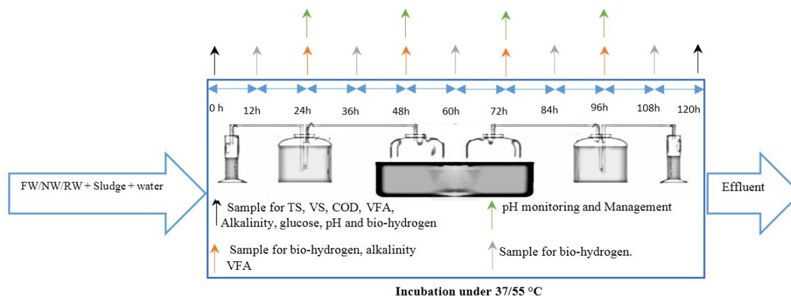
**Figure 1. Schematic diagram of experimental setup.**
