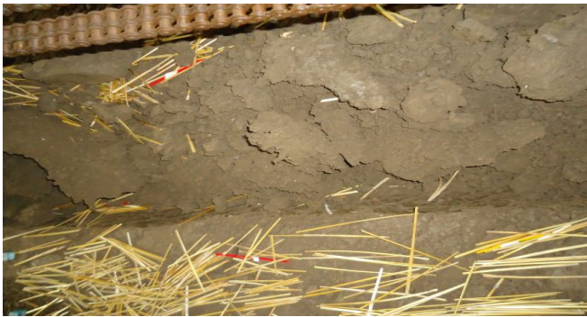
Figure 5. Soil disturbance pattern after single pass of disc tillage tool
