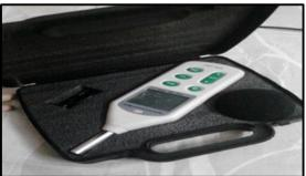
Figure 1.1 Digital Sound Level Meters
