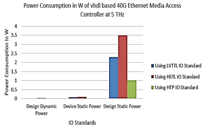
**Fig. 4: Overall Power Ingesting for 40G EMAC Operated at 5 THz**
