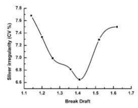
Figure 2 Effect of Break draft short term sliver unevenness
