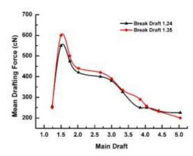
Figure 3 Effect of draft in front drafting zone with different break drafts.
