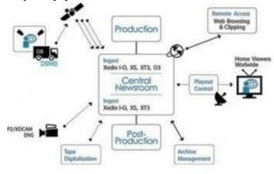
Figure 1: Block Diagram of Operational Department in a Digital Television Channel
