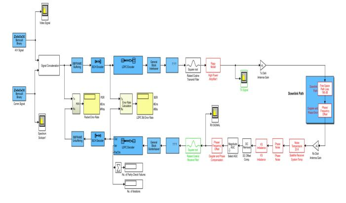
Figure 3: DVB-S2 Broadcast System with a communication channel
