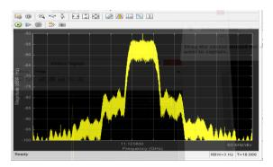
Figure 8: Received Signal Power Spectral Density (PSD)
