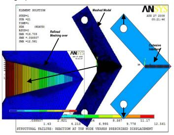
A comparative plot has been presented below which shows the load displacement graphs obtained by running the simulations through ANSYS with the change of the corner radius. The difference is obvious where the required cohesive force need to break the specimen apart is much higher as the corner radius is increased.
