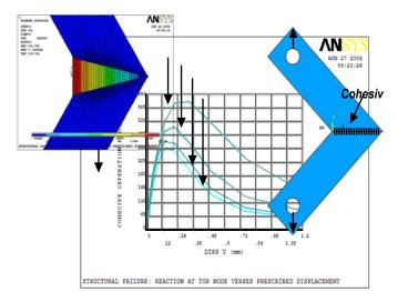
FAILURE PREDICTION AND CRACK PROPAGATION WITH STRESS CONCENTRATION USING COHESIVE ZONE FINITE ELEMENT ANALYSIS
