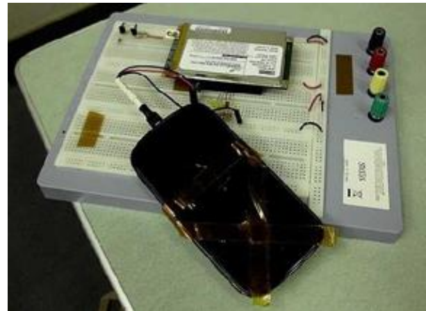
Fig 11 : The Development Model (DM) of PhoneSat-1, operated by NASA [5]
