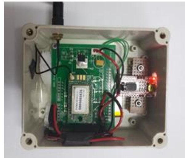
Fig 8 : The Zigbee transmitter, with implementation of changes in terms of circuits' disposition and mechanical strengthening [5]
