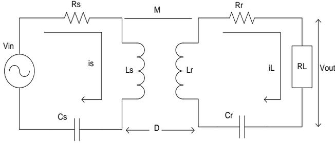
Fig. 1 Magnetic Resonance Coupling Model
