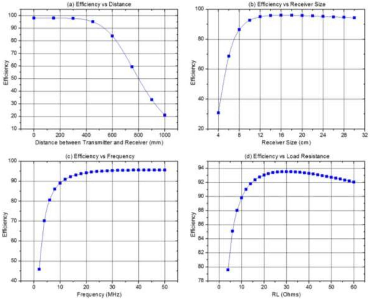
Fig. 3 Parametric Relationship of Magnetic Resonance Coupling
