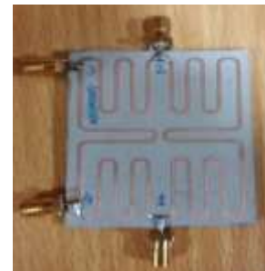
Fig 4. Rate-Race hybrid coupler
