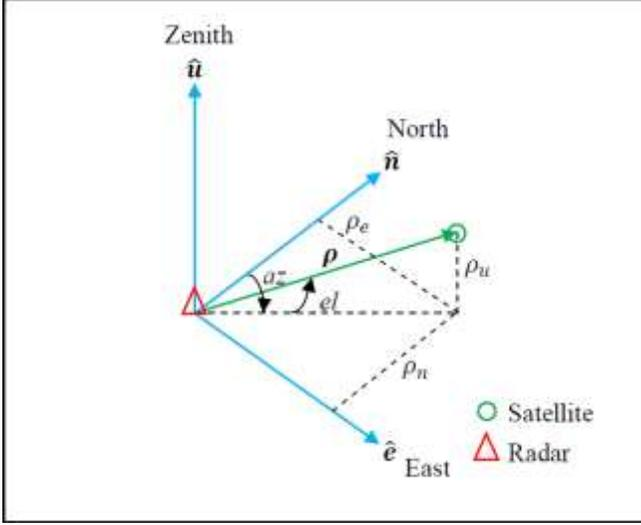
Fig. 3. Topocentric Coordinate System for RADAR Observations
