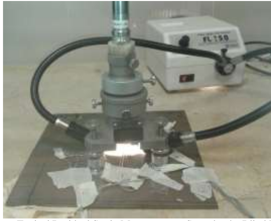
Fig.6. Typical Residual Strain Measurements Setup by the Blind Hole Drilling Method
