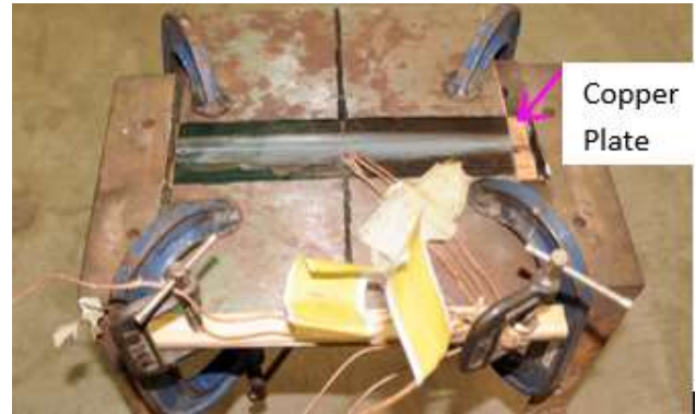
Fig. 1. Experimental Setup for Welding (Specially designed welding jig for clamping)
