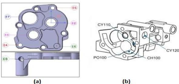
Fig. 7. (a) Oil Pump Cover (b) Oil pump Body Variant
