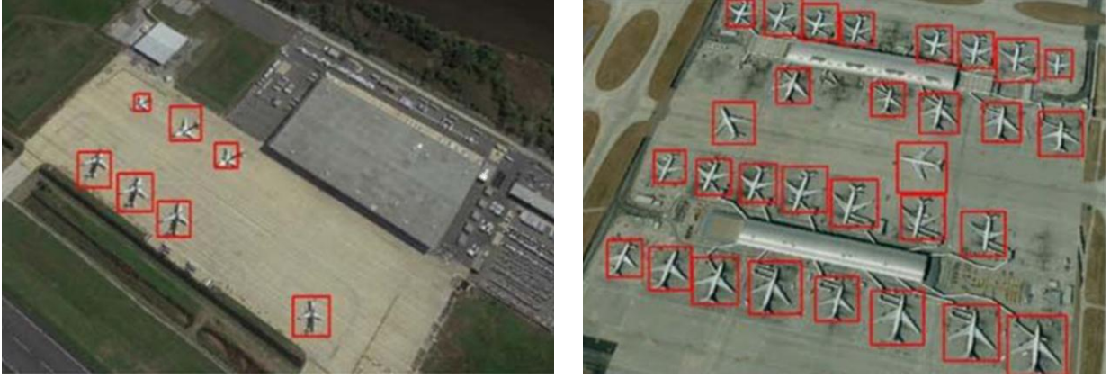
Figure 5. Results of the proposed target detection system on some test images from the aircrafts dataset.
