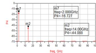
Figure 20: Conversion Loss of above circuit (16.727dB)
