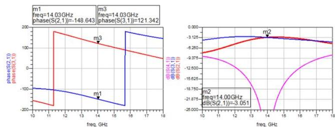
Figure 25: Frequency response of 90° Hybrid at 14GHz
