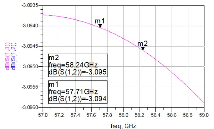
Figure 22: Frequency response of Wilkinson divider at 58GHz (insertion loss)
