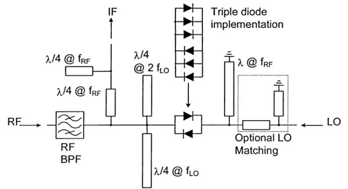
Figure 5: A 4x Subharmonic Mixer topology using triple diode implementation [21]
