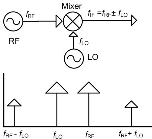
Figure 3: Basic operation of Mixer
