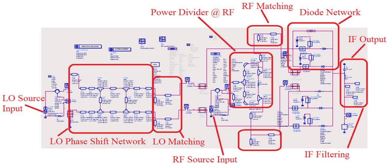
Figure 28: Microstrip realization of 4x Subharmonic Mixer with LO at 14GHz, RF at 58GHz and IF at 2GHz
