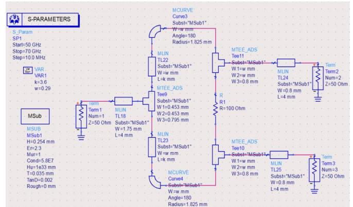
Figure 21: Microstrip circuit of Wilkinson divider at 58GHz
