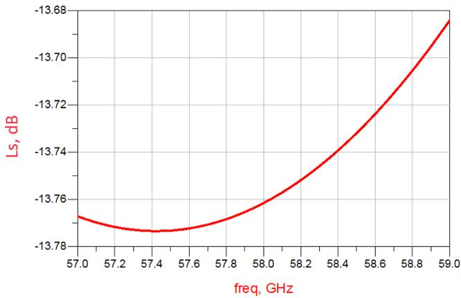
Figure 32: Conversion Loss of the Mixer
