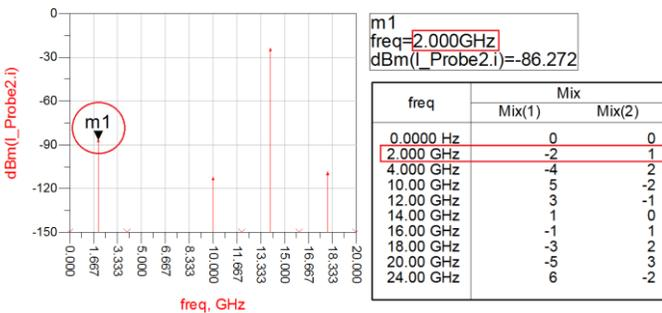
Figure 18: The mixing product at 2GHz is generated by the 2xsubharmonic action, where LO is at 14GHz and RF at 30GHz
