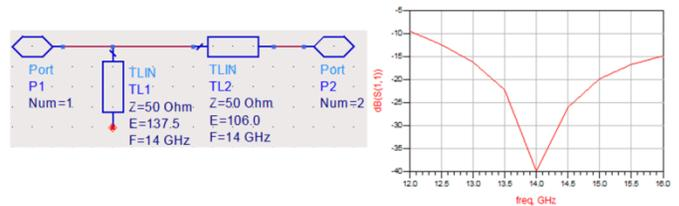
Figure 27: Matching network with frequency response at 14GHz
