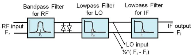
Figure 4: Block diagram of a basic 2x Subharmonic mixer
