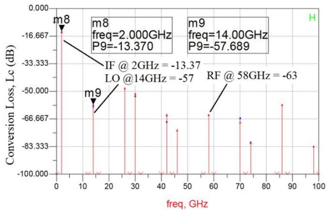
Figure 31: Conversion Loss for m=2 after optimization referred to 0dBm RF Power
