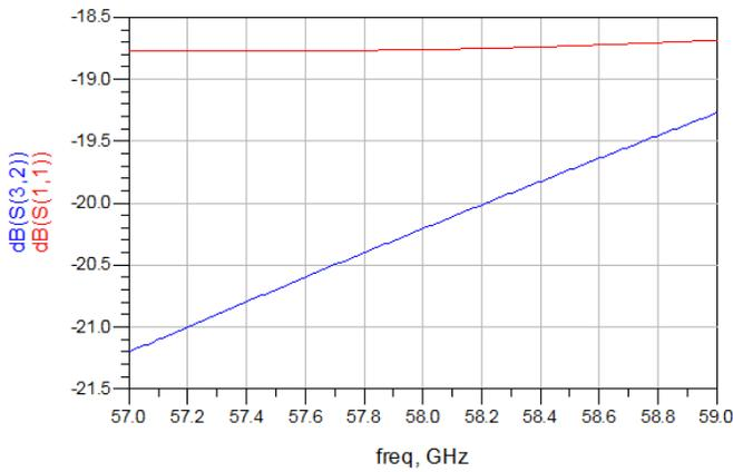
Figure 23: Frequency response of Wilkinson divider at 58GHz (Output ports Isolation & Return loss of input port)
