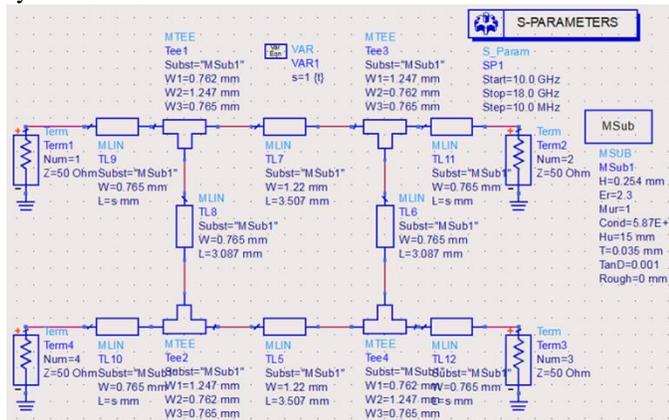
Figure 24: Microstrip realization of a 90° Hybrid at 14GHz
