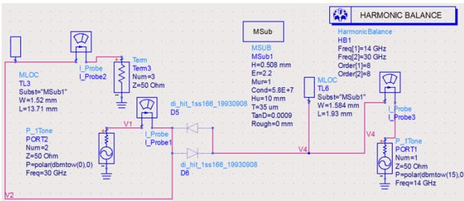
Figure 17: Schematic for a 2x Subharmonic mixer
