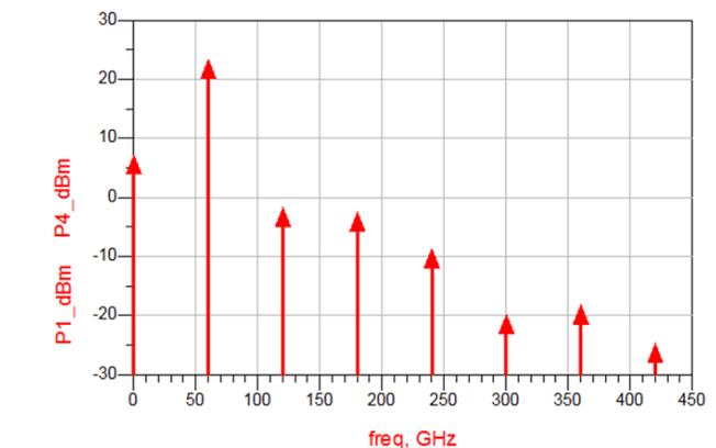
Figure 14: Output power of a diode for 60GHz input
