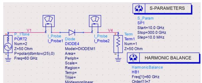
Figure 13: Simulation of non-linear behavior of a typical diode
