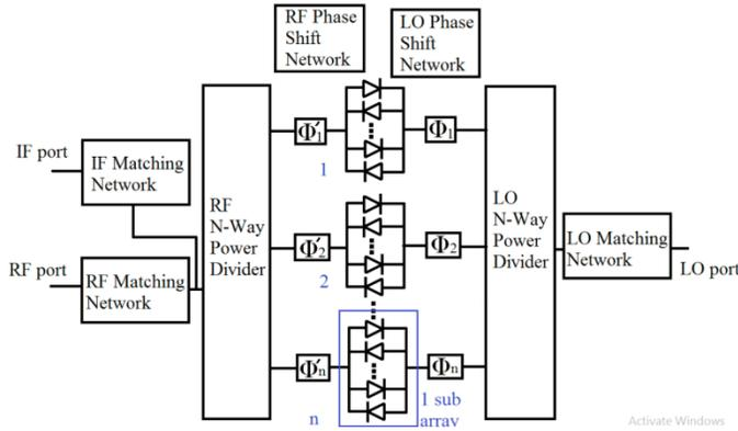
Figure 9: A generic high order Subharmonic Mixer configuration using multiple antiparallel diode pairs
