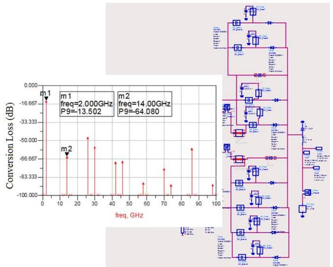
Figure 30: Conversion Loss ( m=3 results in better conversion efficiency than for m=2) referred to 0dBm RF Power
