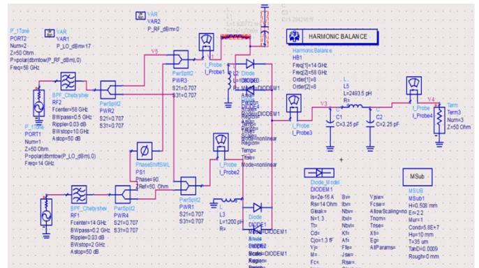
Figure 19: Schematic diagram of a 4x Subharmonic mixer (RF=58GHz, LO=14, IF=2)
