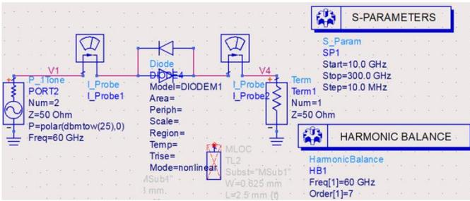
Figure 15: Circuit for simulation of behavior of a typical APDP
