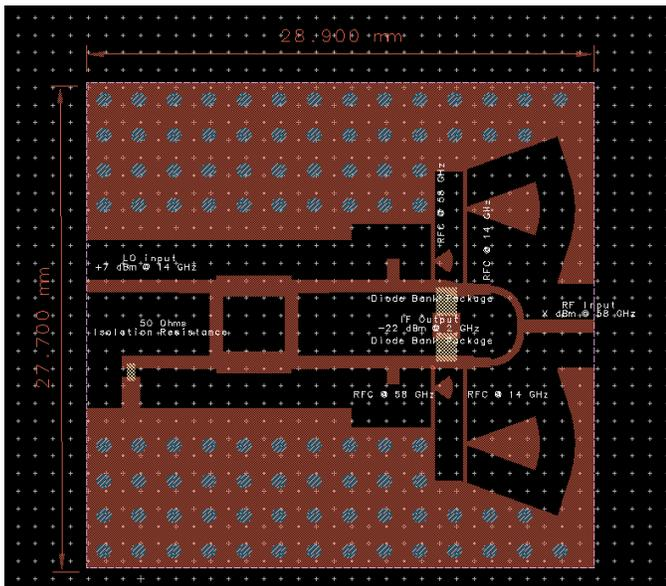
Figure 34: Final Layout of the 4x Subharmonic mixer
