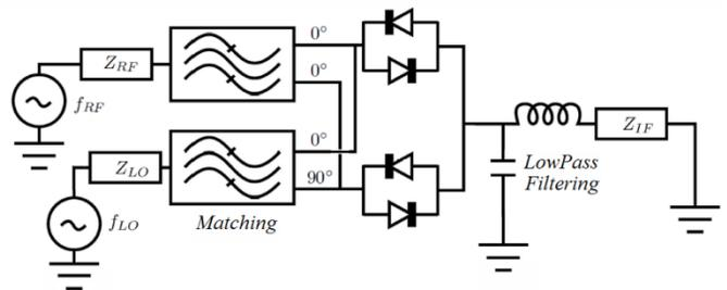
Figure 6: A 4x Subharmonic Mixer topology using 2 APDPs [18]
