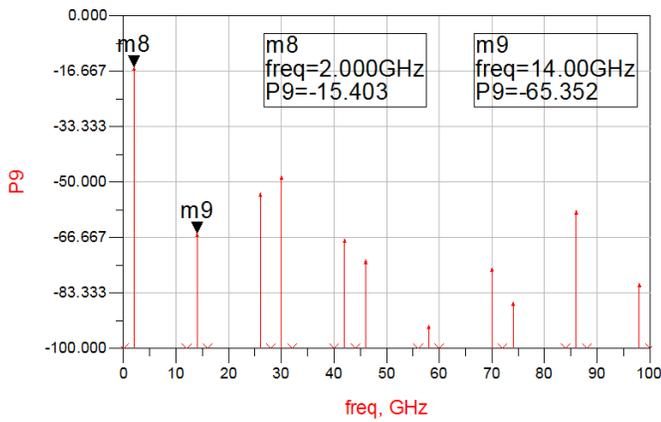
Figure 29: Conversion Loss of 4x Subharmonic mixer referred to 0dBm RF Power
