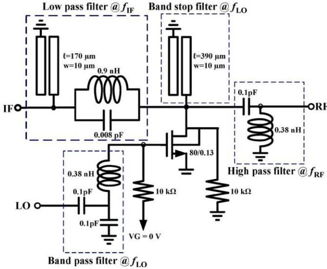
Figure 8: Schematic of 2x SHM [23]
