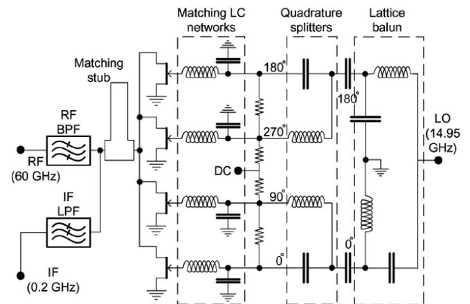
Figure 7: A 4x Subharmonic Mixer topology using transistors [22]
