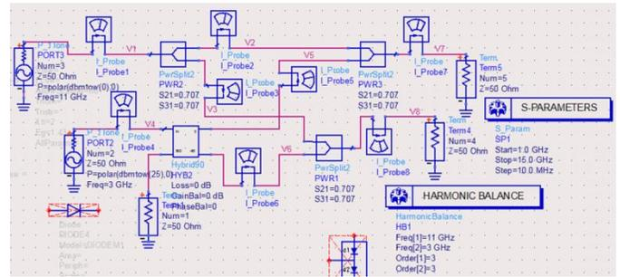
Figure 11: The exemplary linear circuit for a typical Subharmonic mixer
