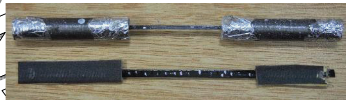
Fig. 7. Epoxy impregnated specimens of unidirectional carbon fiber tows
