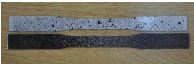
Fig. 5. Two types of speckle patterns with white and black background are shown. As long as the speckle size remains the same, the choice of background color does not affect the correlation
