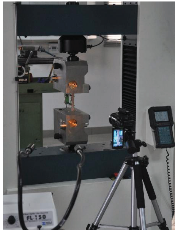
Fig. 2. Experimental setup for uniaxial tensile tests. The digital camera is positioned in such a way that the area of interest remains in the frame. Halogen lamps are visible in the foreground illuminating the specimen surface with controlled light intensity suitable for correlation.
