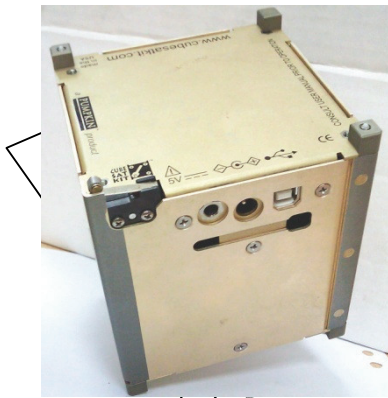
Figure 3 - ICUBE-1 IU structure
