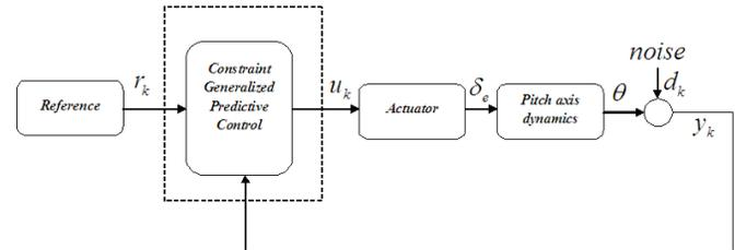
Figure 2 - Complete system block diagram
