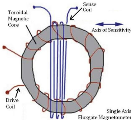
Figure 3 - Arrangement of Excitation and Sense Coil of Magnetic Core
