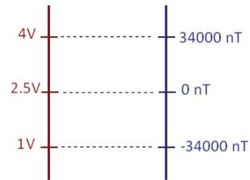
Figure 16 - Field corresponding to output Voltage
