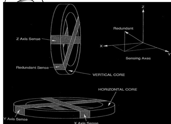
Figure 5 - Sense coils with redundant axis configuration
