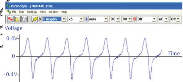
Figure 12 - Sense coil output at 10kHz frequency (-ve field)
