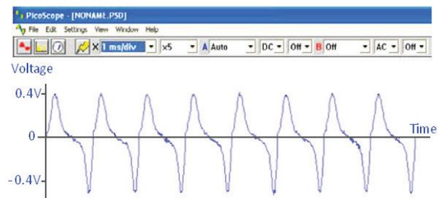
Figure 11 - Sense coil output at 10kHz frequency (+ve field)
