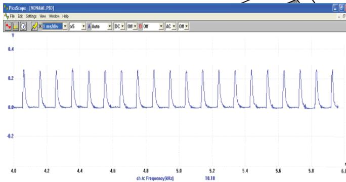
Figure 14 - Sampled Sense waveform (+ve field) 50% of the waveform was not sample
