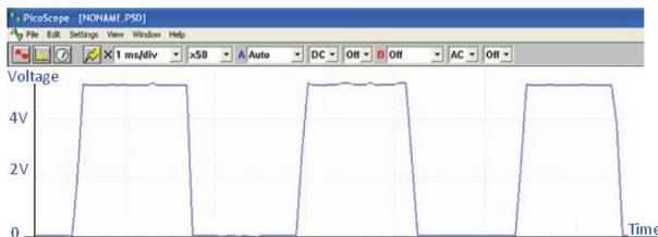
Figure 8 - Excitation output 20kHz
