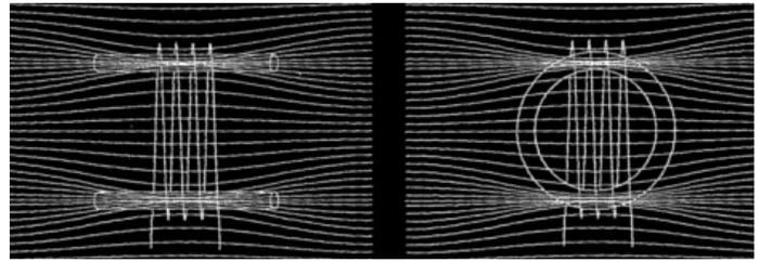
Figure 4 - Flux line for dual core and ring core magnetometer
