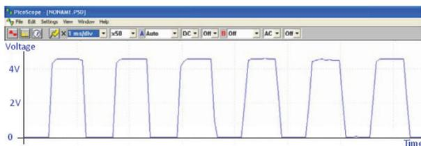
Figure 7 - Excitation output 40kHz
