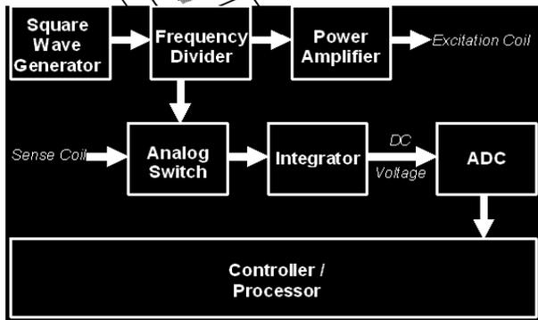
Figure 6 - Block Diagram of Fluxgate Magnetometer
