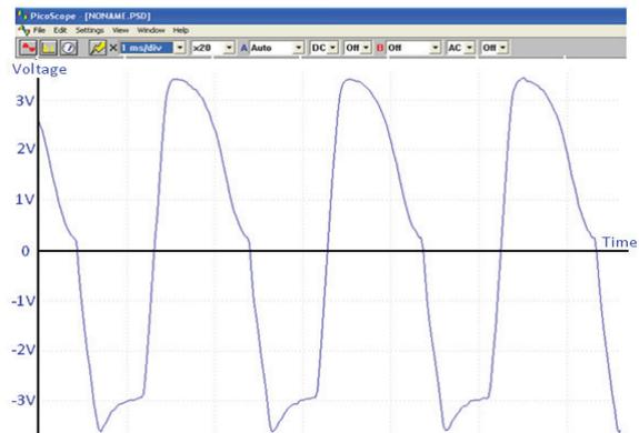
Figure 9 - Excitation output after connecting coil
