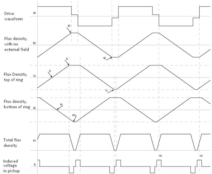
**Figure 1 - Induced Voltage in pickup coil due to mutual induction of excitation and sense waveforms**
