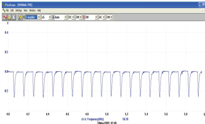
Figure 15 - Sampled Sense waveform (-ve field) 50% of the waveform was not sampled
