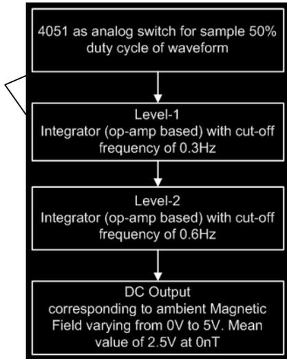
Figure 13 - Block Diagram of Sense Circuit
