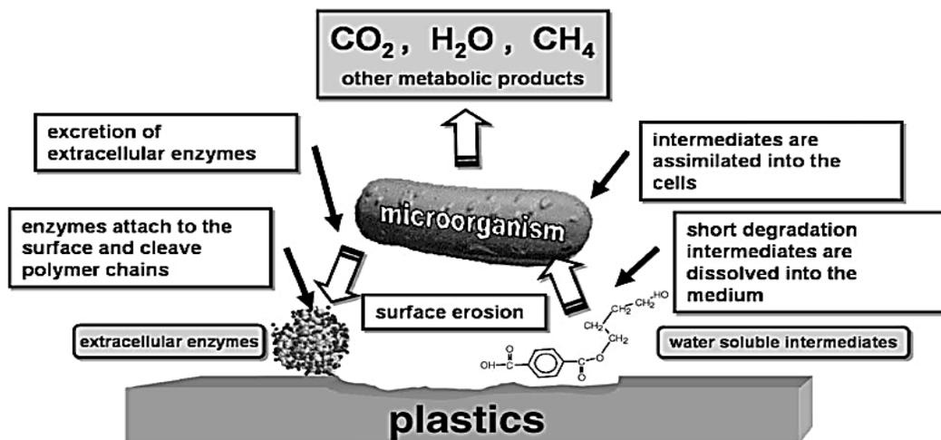
Fig. 3. The general mechanism of enzymatic catalyzed hydrolytic polymer degradation (Mueller, 2006).
