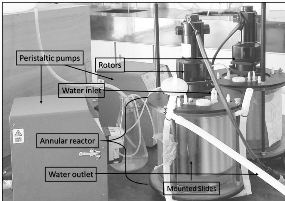
Fig. 1. Experimental set up of annular reactors for biofilm formation in pilot-scale lab showing 2 annular reactors, peristaltic pumps, Inlet, and outlet water sources.
