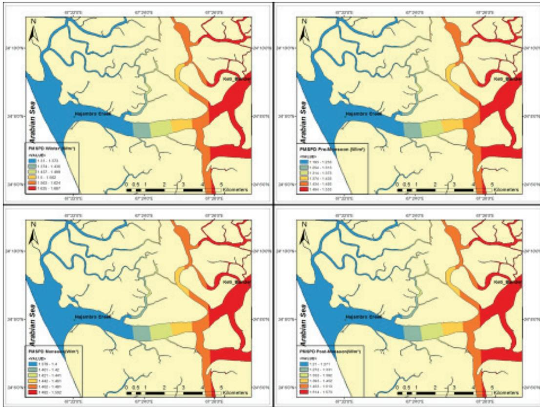
Fig. 6. PPD model for four seasons representing potential mean spring power density (in  $W/m^2$ )
