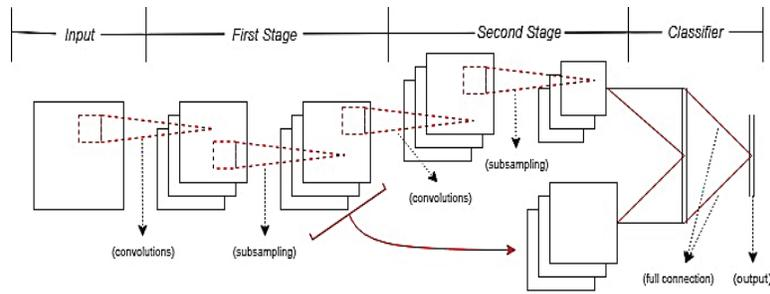
Fig. 4. A typical CNN block scheme [10]
