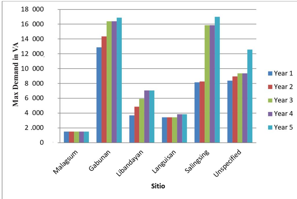
Fig. 2. Comparison of Load Demand Profile for 5 yr.
