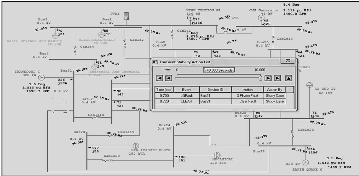
Fig. 7. Transient stability analysis of UET Microgrid
