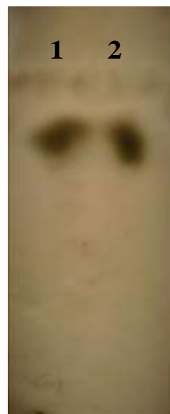
Figure 7. Thin-layer chromatography (TLC) of hydrolysis products of pullulanase from pullulan (lane 2) and standard maltotriose (lane 1)
