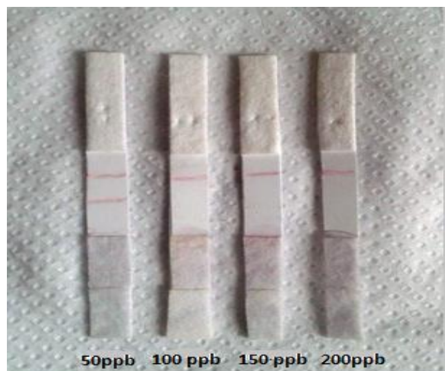
Figure 10. Strips showing negative (at 50 ppb) and positive results at various concentrations (100, 150 and 200 ppb)
