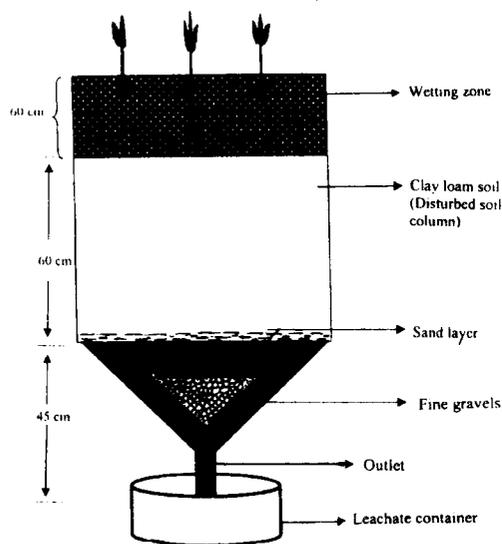
FIGURE 1. SCHEMATIC DIAGRAM OF COLUMN LYSSIMETERS DESIGN AND INSTALLATION
