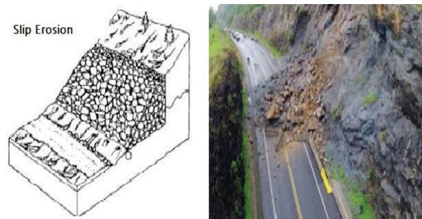
Fig. 6. Slip erosion may also culminate in landslides, which can damage buildings and roads.
