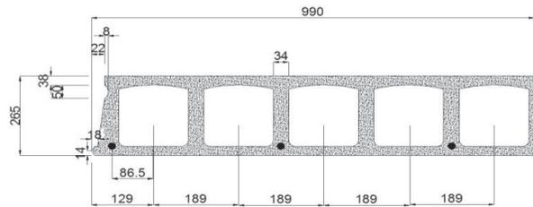
Fig. 2. Cross section of hollow core slab with 265 mm depth
