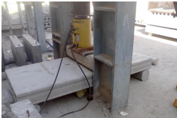
Fig. 3. Testing arrangement for slabs in flexural loading
