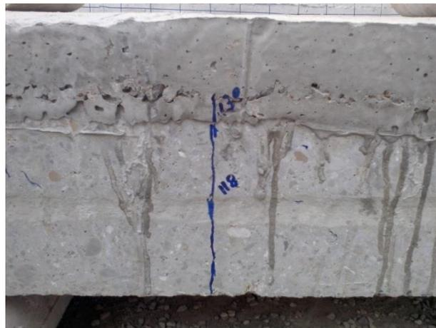
**Fig. 8.** Crack pattern of slabs under flexural loading
