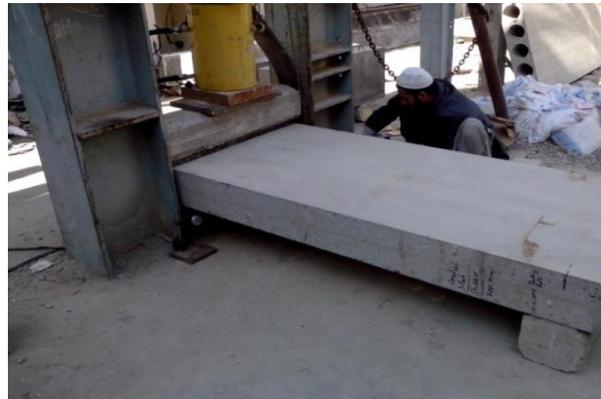
Fig. 4. Testing arrangement for slabs in shear loading
