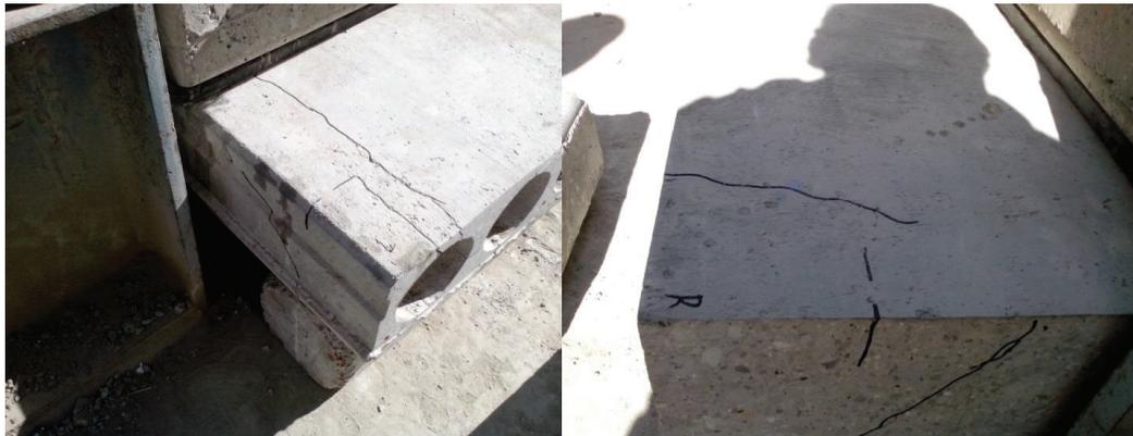
(a) Crack patterns under shear loading for 200mm depth slab from side
