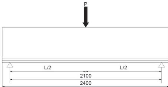
Fig. 5. Schematic diagram of flexural test
