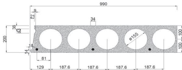
Fig. 1. Cross section of hollow core slab with 200 mm depth
