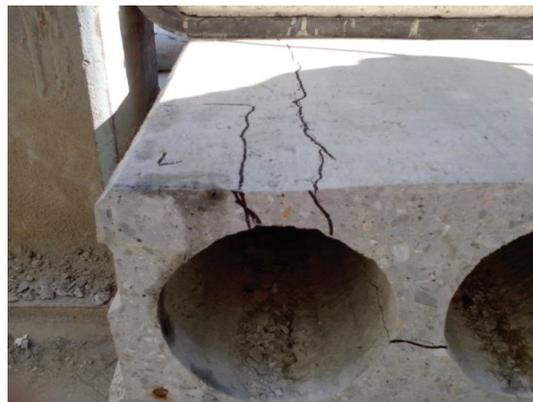
(c) Crack patterns under shear loading for 200mm depth slab from front
