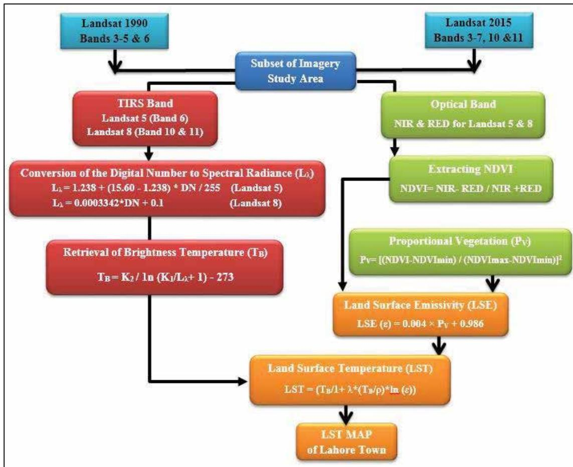
Fig. 2. Overall Methodology and Process of Land Surface Temperature Retrieval
