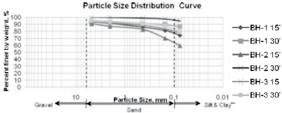
Fig. 9. Sieve analysis of soil samples recovered from boreholes (ASTM-D422-63 method)
