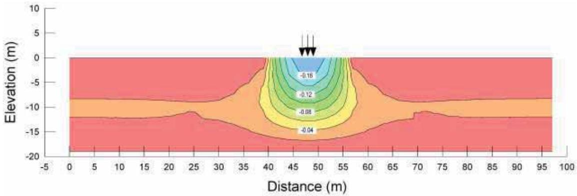
Fig. 10. Settlement analysis for existing soil beneath building
