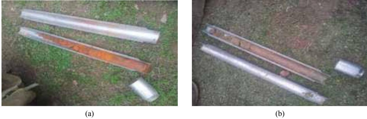
Fig. 7. Soil Sample obtained from BH-3 at (a) 1.8m and (b) 7.6m depth
