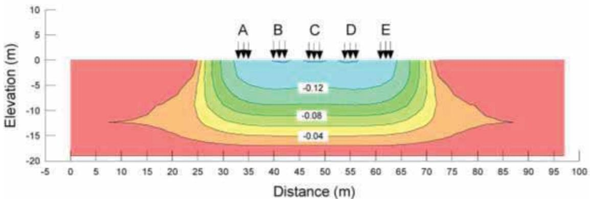
Fig. 12. Settlement analysis of five (5) footings with recommended soil replacement of 6 m
