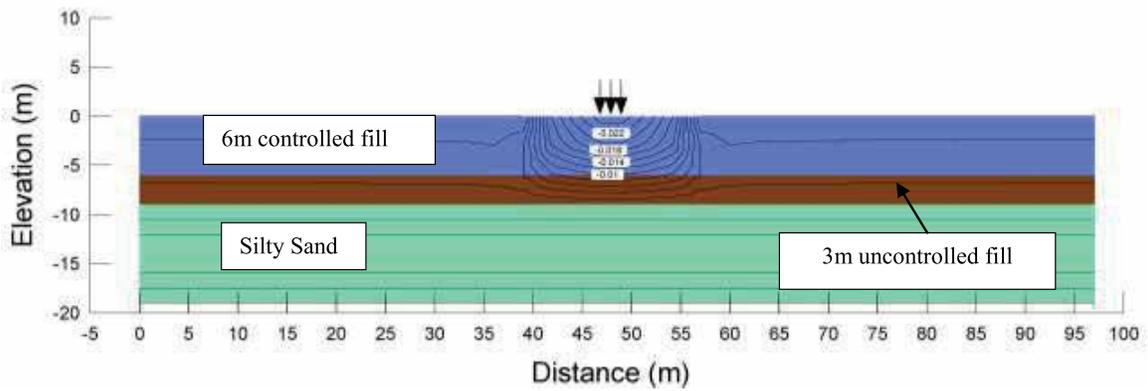
Fig. 11. Settlement analysis with recommended soil replacement of 6 m
