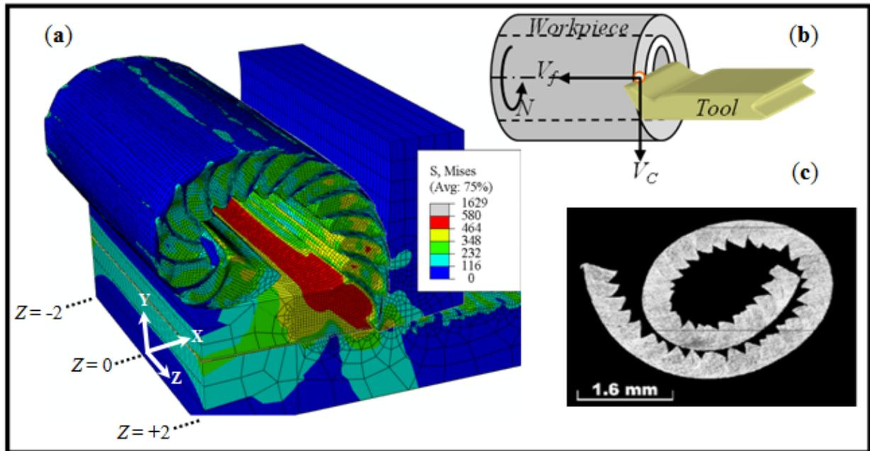
Fig. 2. Chip morphology for orthogonal turning for  $V_c = 800$  m/min,  $f = 0.5$  mm/rev,  $a_p = 4$  mm.
