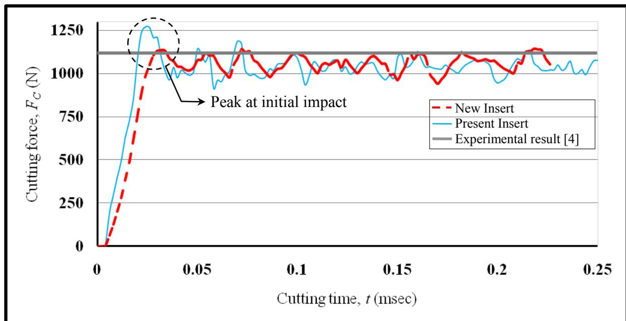
Fig. 6. Plots of cutting forces for  $V_C = 800$  m/min,  $f = 0.5$  mm/rev,  $a_p = 4$  mm.
