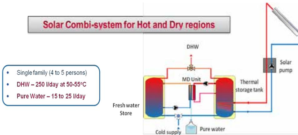
Fig. 1. Prototype design of plant setup [13].
