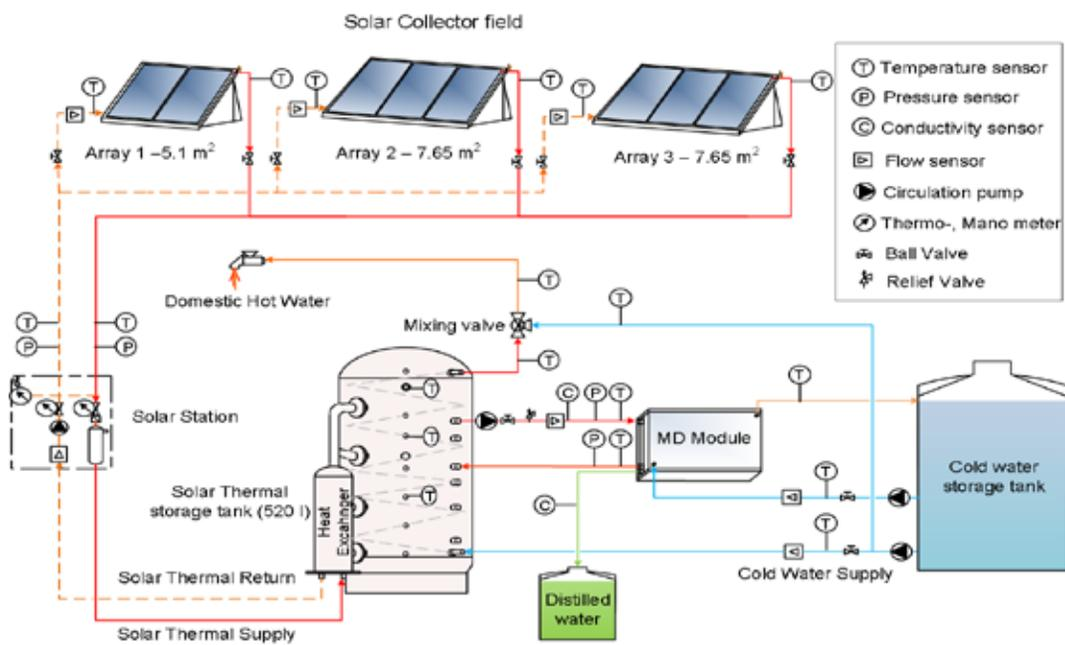
Fig. 3. Integrated SDHW-MD Onsite Setup [13]
