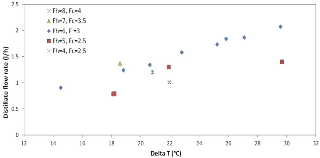
Fig. 11. Distillate flow rate vs Delta T (hot in temperature-cold in temperature).
