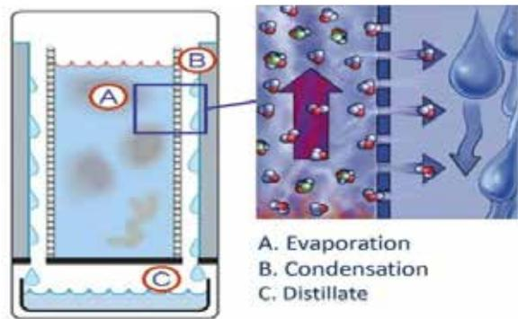
Fig. 2. Air Gap Membrane Distillation Technique [13].
