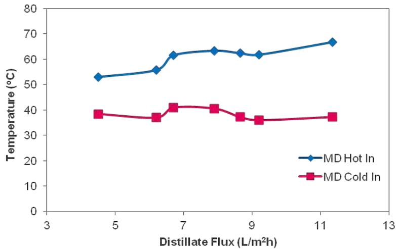
Fig. 12. MD hot and cold feed temperatures vs. distillate flux.
