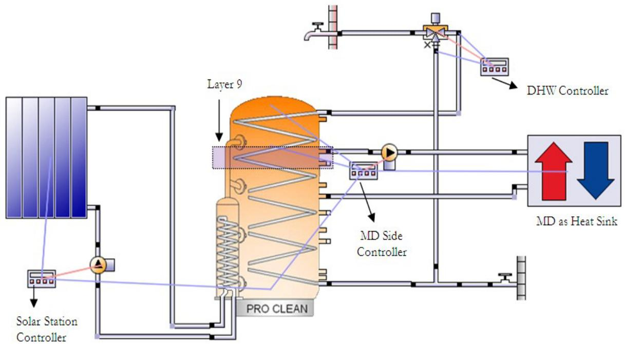
**Fig. 6.** PolySun simulation model SDHW-MD system [13].
