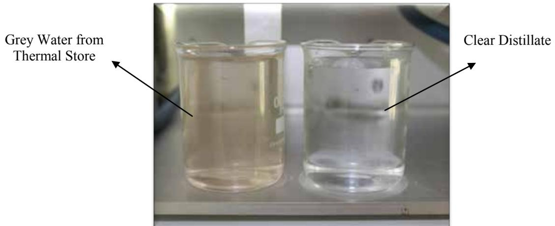
Fig. 10. Samples of grey water and clear distillate.
