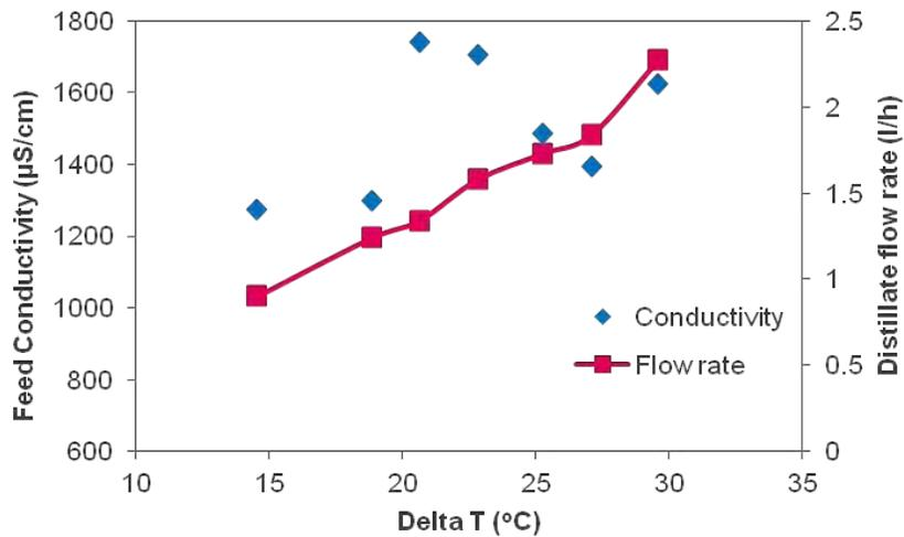
Fig. 13. Feed water conductivity vs. distillate flux.
