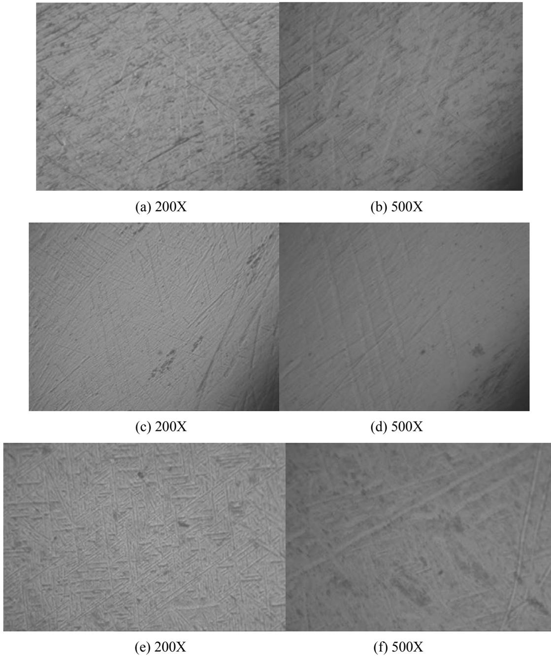
**Fig. 3.** The microstructure of solution treated  $\text{Ti}_{91}\text{Al}_5\text{V}_4$  (a, b),  $\text{Ti}_{90.5}\text{Al}_{5.5}\text{V}_4$  (c, d) and  $\text{Ti}_{89.5}\text{Al}_{6.5}\text{V}_4$  (e, f).
