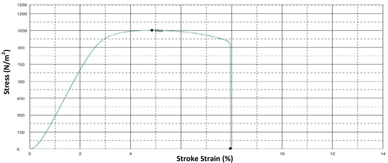
Fig.8 (b). Tensile testing graph for  $Ti_{89.5}Al_{6.5}V_4$ .
